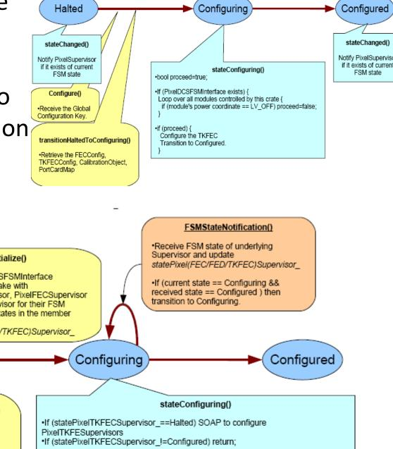
Retrieve the DetectorConfiguration, the NameTranslation and the CalibrationObject. Retrieve the TKFECConfig, PortCardMap and PortCard if there exists a PixelTKFECSupervisor If (statePixelFECSupervisor\_==Halted) SOAP to configure PixelFECSupervisors Retrieve the FECConfig if a PixelFECSupervisor exists Retrieve the FEDConfig if If (statePixelFEDSupervisor\_==Halted) SOAP to configure PixelFEDSupervisors
