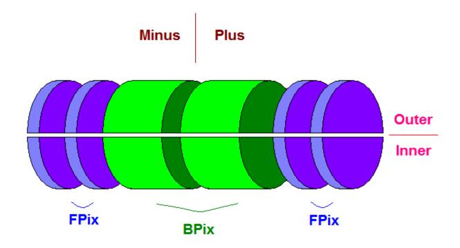
→ The Pixel Detector is partitioned into 8 segments:
