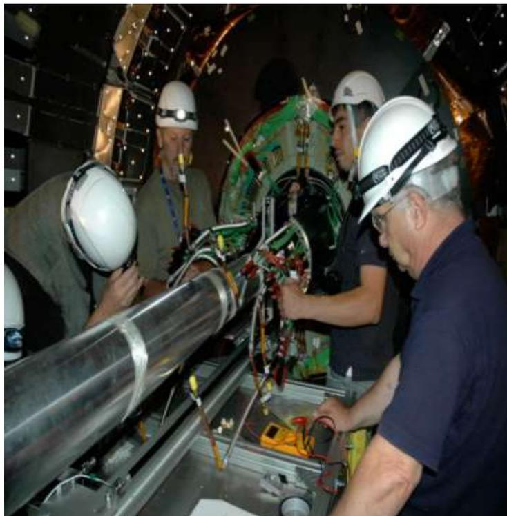
Synchronous insertion of the inner and outer half-cylinders.
