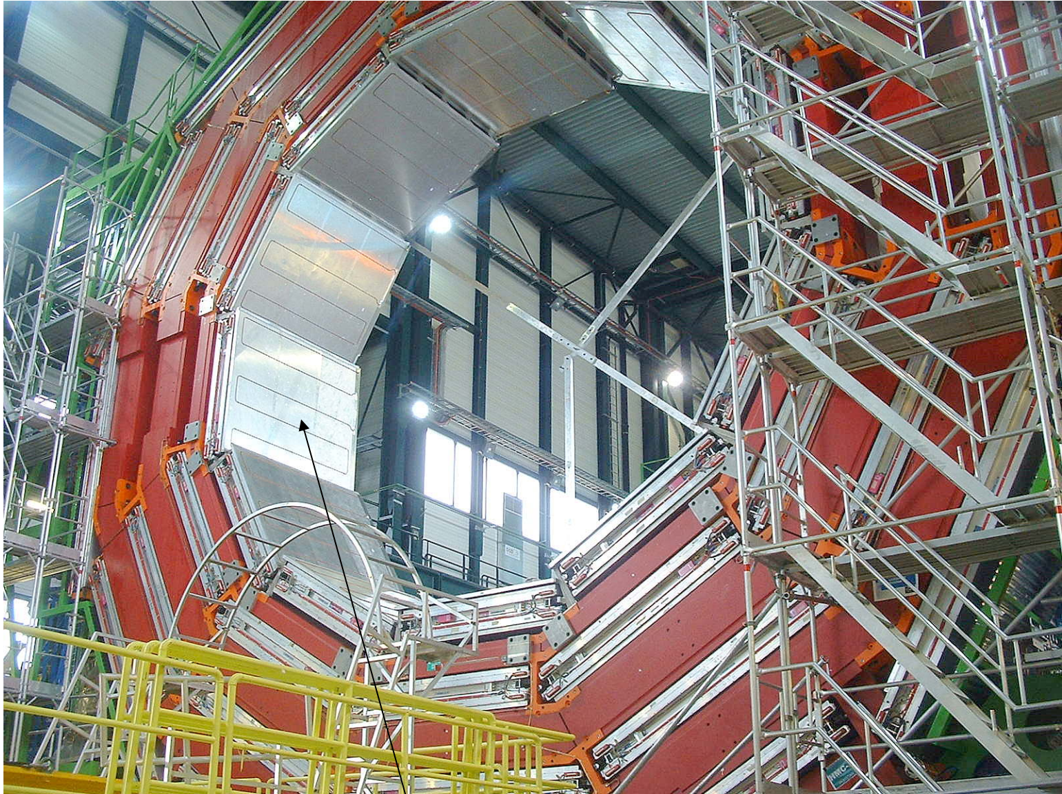
Drift tubes to detect muons
