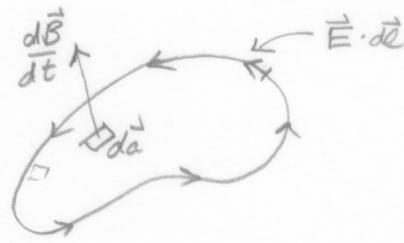
$$\int_S ((\nabla \times \vec{E}) \cdot d\vec{a}) = - \int_S \frac{\partial \vec{B}}{\partial t} \cdot d\vec{a}$$
