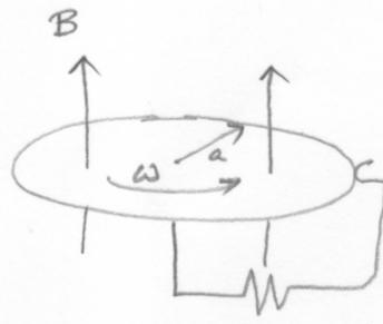
$$\begin{aligned} f_{\text{mag}} &= qvB \\ &= q \omega B \\ \therefore V_{\text{emf}} &= \int_0^a f_{\text{mag}} \cdot da = \oint B \omega \int_0^a r dr \\ &= \frac{q B \omega a^2}{2} \end{aligned}$$
