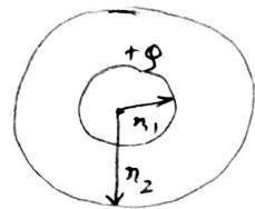
Two concentric spherical conducting shells.
